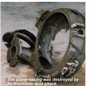
These photos are of a pump from a gold mine which was repaired by an ENECON Fluid Flow Systems Specialist in Australia.
