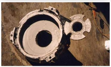
CeramAlloy CP+ was used to rebuild all damaged surfaces.
