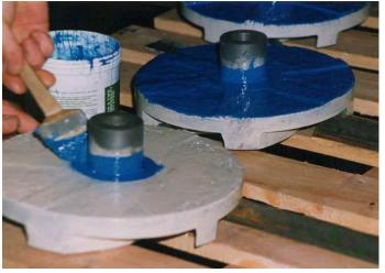
in suspension. Obviously, this is a very aggressive wear condition so the mine's engineers are absolutely delighted with the performance of the FLEXICLAD DuraTough in this highly abrasive fluid flow environment.
