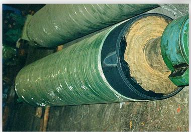
These rubber rollers run against stone rollers and had become damaged due to a misalignment problem.
