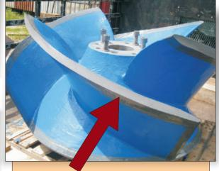
**CeramAlloy CL+AC** used to protect the impeller's edges.
