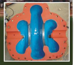
and this pump was expertly repaired and protected from future erosion-corrosion damage in just a few days for less than 1/3 the cost of a new pump.
