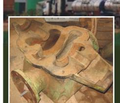
This Brazilian paper mill stock pump was severely damaged after 12 years of continuous use. The mill's engineers sent the pump out to two separate pump repair companies who advised that this pump was "unrepairable" and suggested replacement as the only viable option.
