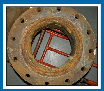
The component is a 14" diameter, cement lined, spool piece that is mounted between a large strainer and an isolation valve on the service water system at a nuclear power station. During a refueling outage, this spool piece was removed to allow for maintenance on an adjacent component. The deteriorated condition of the piece was unexpected. The cement lining was severely eroded as were the inside diameters of both the inlet and outlet flanges.
