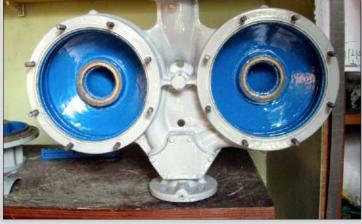
This hard water pump at a hospital in Chile was only averaging a few months in service before maintenance would have to be performed to repair deep erosion / corrosion damage.
