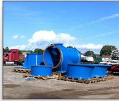
A major U.S. nuclear power plant chose The circ. pump components were **ENECON** to supply turn-key services to install CeramAlloy CL+AC on 12 massive circulating pump (circ. pump) casings. The plant's engineers felt that the performance of CeramAlloy on the circ. pump impellers, (reference MT-114) in a demanding brackish water environment was proof enough that CeramAlloy should be used to protect 12 circ. pump casings during a system overhaul.
