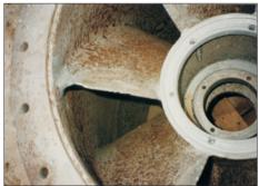
Severe erosion/ corrosion damage to pumps...
