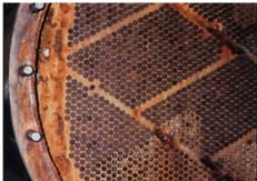
Severe erosion/corrosion damage to chillers, tube sheets, water boxes, and flange faces...
