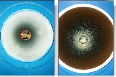
A U.S. based aluminum ferry boat manufacturer used ENECON's *METALCLAD CeramAlloy HTL* to protect exhaust tubes on four new ferry boats. A combination of high temperature exhaust and salt water causes these aluminum tubes to corrode very quickly.
