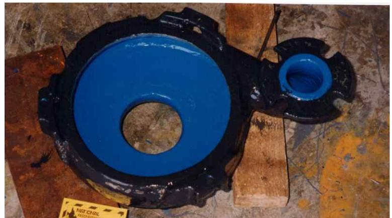
*CeramAlloy CL+ was used to protect all internal surfaces.
