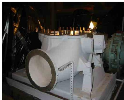
The resurfaced pump will provide many additional years of service and improved efficiency.
