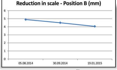
Scale measurements at 2 different positions show reductions in scale over time.
