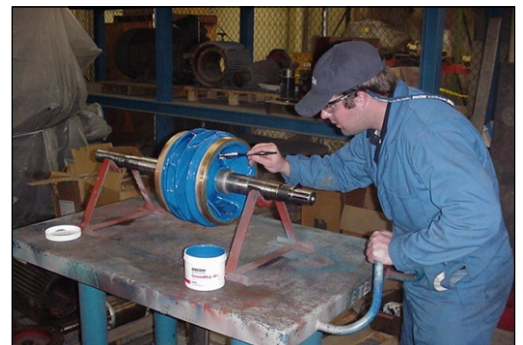
CeramAlloy CL+AC being applied
