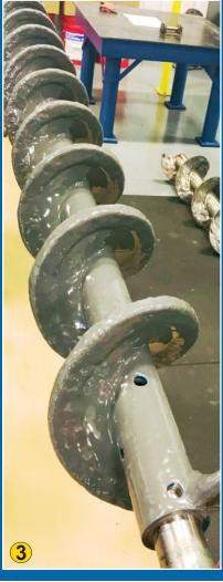
Engineers at an activated carbon plant in the southern US were in need of an abrasion resistant coating for the pushing side / cutting edge of several new horizontal screw conveyors.
