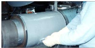
*METALCLAD® DurAlloy®* is a two-component, 100% solids, multi-purpose polymer composite which can be easily machined on a lathe, drilled, tapped, filed, sanded and polished...
