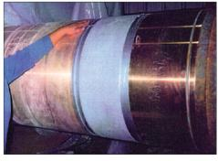
When properly mixed, *METALCLAD*<sup>®</sup> *DurAlloy*<sup>®</sup> is a non-sagging paste which quickly cures to a metal-hard material creating a permanent bond to any rigid surface such as metal, plastic, glass, wood, concrete and more.
