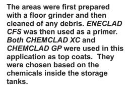
Two coats of CHEMCLAD XC were applied to the containment area containing sulfuric acid tanks. The second containment area has tanks that contain sodium hydroxide. Two coats of CHEMCLAD GP were applied there. Both products provide outstanding chemical resistance to the chemicals they were chosen for.
