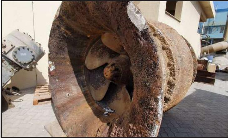
This circulating water pump had been in operation at an electric power plant in the U.A.E. for 30 years. It was opened for the first time and was found to be in poor condition.
