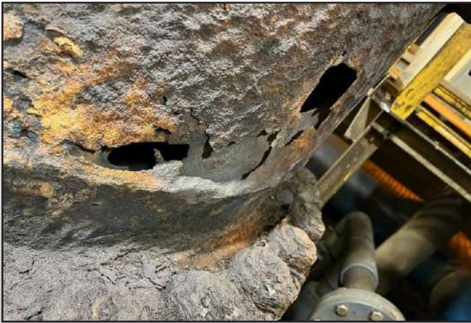
Damage exposed after grit blasting.
