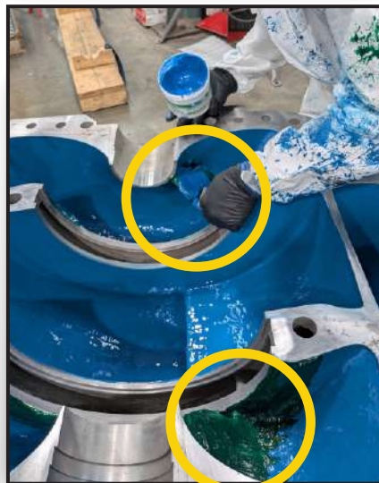
DuraTough DL not overcoated by CeramAlloy CL+AC.
