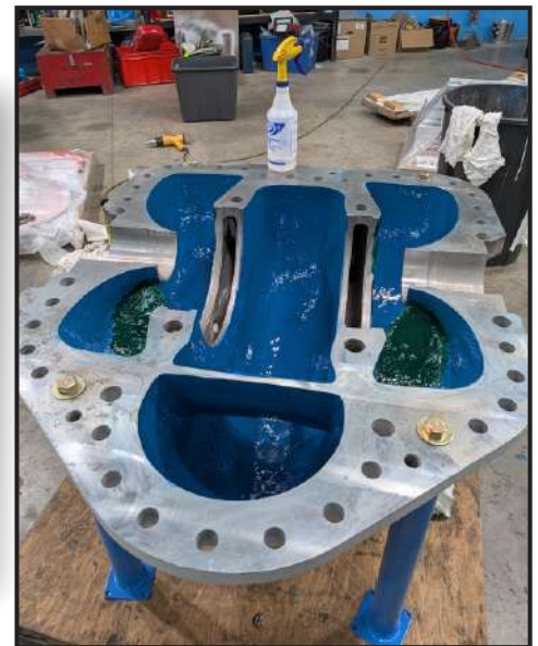
DuraTough DL applied to stop cavitation.
