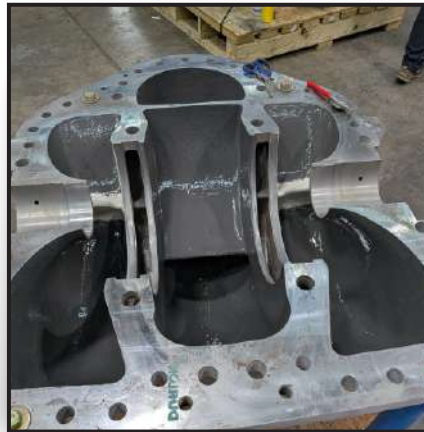
DuraTough DL applied to stop cavitation.
