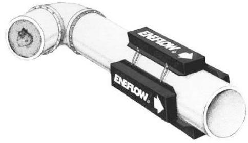
**The Power Cells should be secured firmly around the pipe using the self-locking plastic straps provided. The Power Cells should be orientated with the fluid flow direction as per arrows on the units.**
