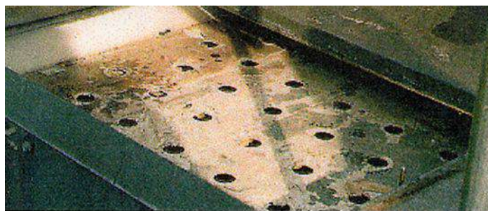
Pool paint peeling on pans poses problems.
