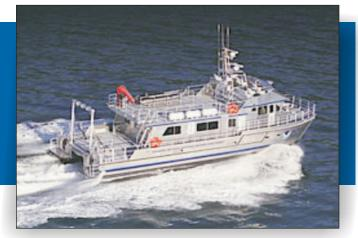
This aluminum hull catamaran is designed to be used as a research platform in one of the National Marine Sanctuaries. The marine engineers wanted a high performance, non-slip deck coating that would provide many years of service. They selected ENECLAD FPS because of its durability and ease of application (no odors or V.O.C's) and ease of cleaning.
