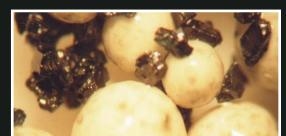
CeramAlloy CBX ceramic microspheres and silicon carbide aggregates.
