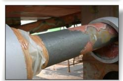
The propeller shafts on this Croatian Naval ship were suffering from severe erosion / corrosion in the areas around the struts and before the propellers. This was due to many years of operation in a harsh salt water environment.
