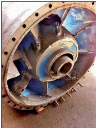
The severely eroded vanes were cut away.
