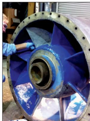
CeramAlloy CL+AC used to coat all surfaces.
