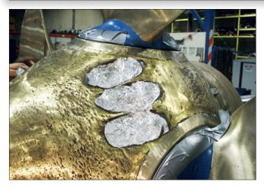
**Controllable Pitch Propellers (called CPP** 'wheels') are used by tug boats, fishing boats and many other commercial vessels. The pitch (angle) of the propeller blades can be adjusted for power, speed and even direction all without changing engine speed. The hub of these propellers, as well as the base of the blades, often suffer severe erosion/corrosion damage. Problem solved.
