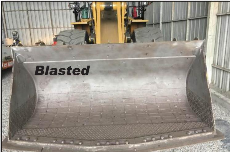
About 80 kilos of CeramAlloy CBX were applied on this bucket. This was the second such bucket completed. The CBX lasted 3 TIMES LONGER than the wear plates – 15,000 hours of operation vs. only 5,000 hours for the wear plates. CeramAlloy CL+AC was used on the rest of the bucket which is not subject to the most aggressive wear.
