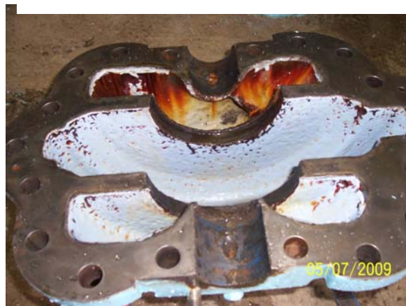
Figure 8-3 After Cleaning with Steel Wool Pad
