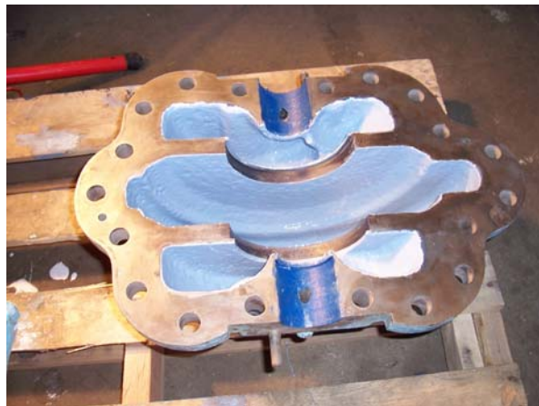
Figure 8-1 Interior of Pump after Coating (2005)
