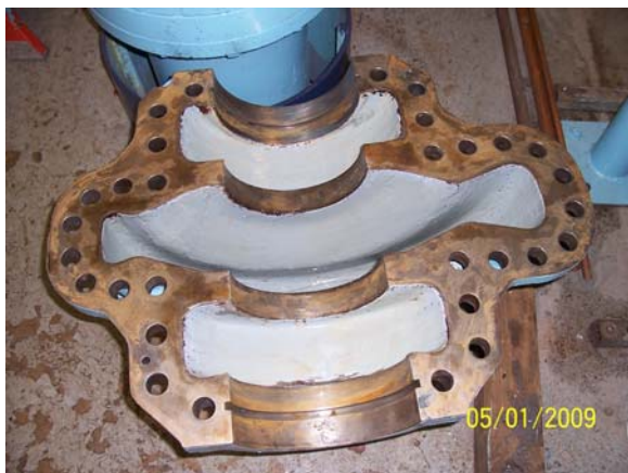
Figure 8-6 Denise Pump after Cleaning with steel wool
