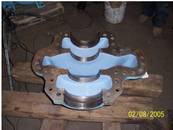
Figure 8-4 Denise Pump Post Coating
