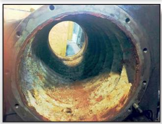
This large air-to-liquid high temperature intercooler, used in the orange juice making process, was severely corroded after years of use.
