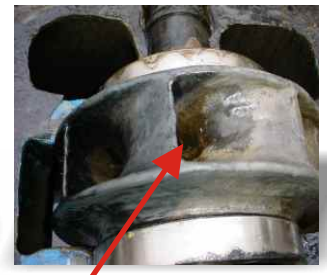
The pump impeller and bottom casing after 9 months continuous duty, showing the DuraTough DL protection of the impeller surface is still in good condition.
